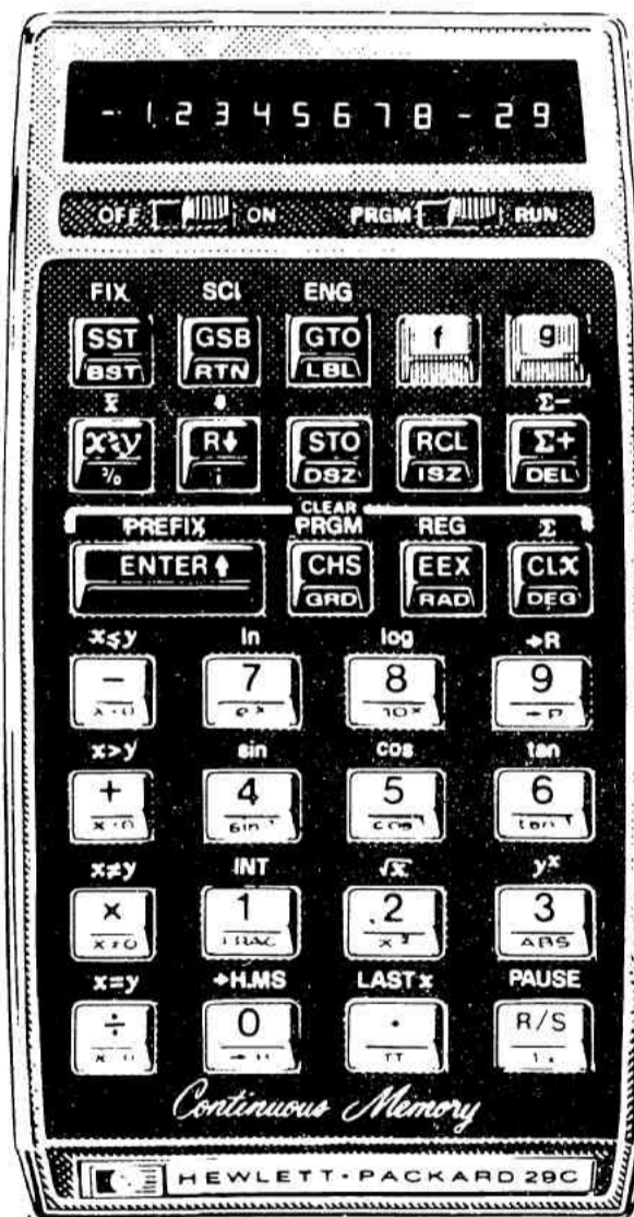
The new HP-29c. Programmable, with continuous memory. 98 programme steps. 30 registers.
